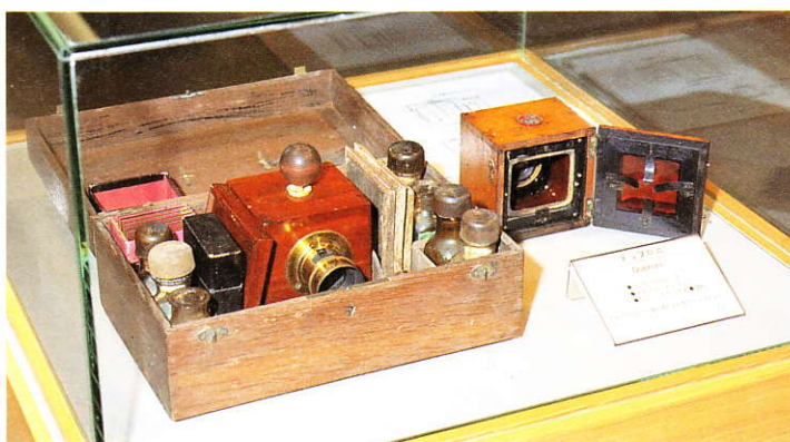
An 1860 Dubroni. One of the first instant cameras. It develops the photos inside the camera body.
